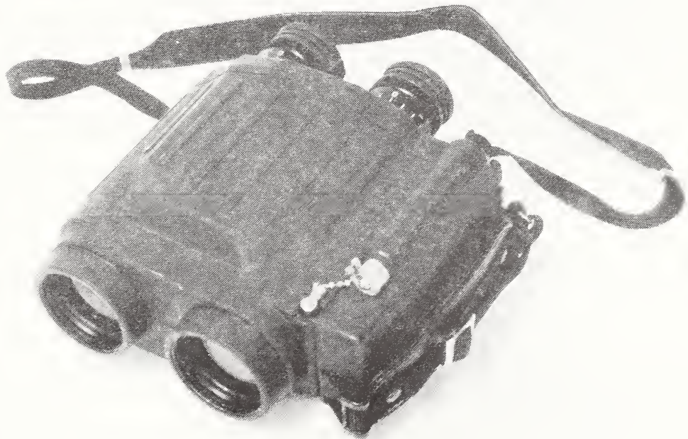
Figure 3. Fujinon Stabiscopes, 14X magnification model.
