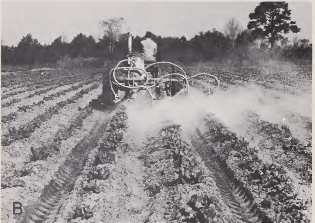
Figure 21. —Tractor-mounted dust machine suitable for applying an insecticide dust for control of caterpillars: A , With cloth hood over outlet nozzles to reduce drift of dust; B , same machine without cloth hood.
