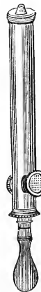
Syringe. Specially designed for applying insecticides on the under side of the leaves.
