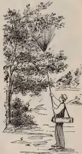
AUTO-SPRAY AT WORK WITH EXTENSION PIPE FOR TALL TREES.
