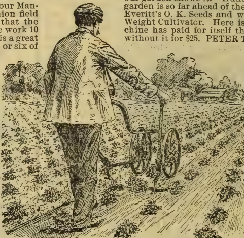
This illustration shows the Man-Weight Cultivator saving a plant that was out of line with others in the row. Notice one drag bar is thrown to the right. Either or both drag bars may be moved to right or left or up or down without changing the direction of the wheels. Perfect adjustability is obtained in these machines.
