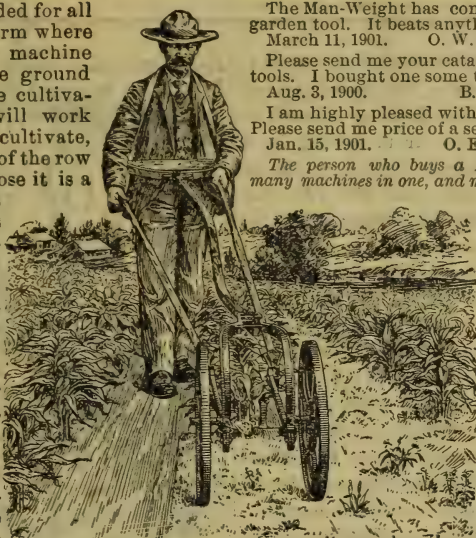
This illustration shows the Man-Weight Cultivator in high stuff. Also it shows the push-bar to allow the operator to walk beside the row instead of astride. (It can be used either way.) This construction is very popular, particularly if the plants are wet. The wheels are 18 inches high. The arch 20 inches. We don't believe you can conceive of a grander labor-saving machine along this line than a Man-Weight Cultivator, if you were to devote the balance of your natural life to the task.
