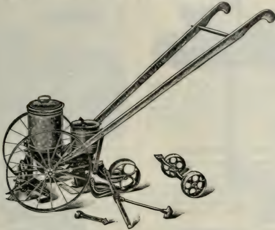
"Iron Age" Combined Fertilizer Distributor, Hill and Drill Seeder.
