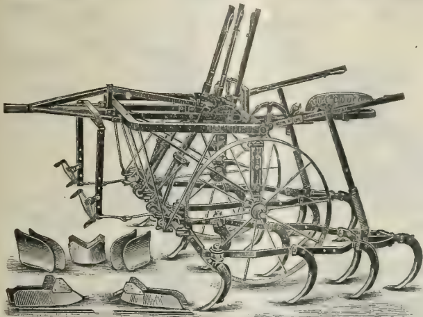
NO. 72 PLANET JR. TWO-ROW PIVOT WHEEL CULTIVATOR, PLOW, FURROWER AND RIDGER.
