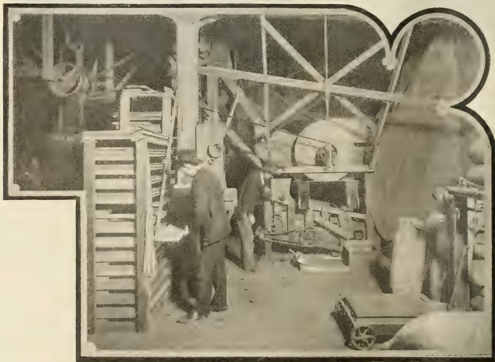
Mill room on third floor. This view shows one of our high speed, dustless Seed Separators with a capacity on most Seeds of 1,000 bushels per day. These immense double suction fans have a speed of six hundred revolutions a minute. They can be adjusted so delicately that they will remove chaff or foreign seed, ranging in weight from one pound to sixty pounds to the bushel. The seed passes from this Separator into immense seed bins from whence the seed is spouted for sacking to any floor in the building. This floor is also used for storing Onion Sets, and the spring season each year finds several thousand bushels stored in special Onion Set crates which keep them in perfect condition until ready for shipment.
