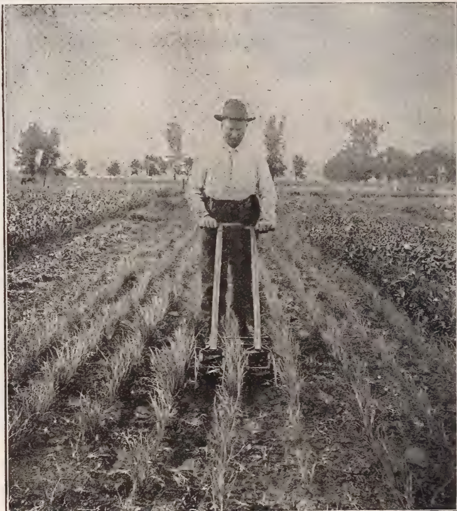
A Double Barker Consists of Two Single Machines Bolted Together. See Description
