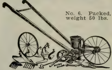
No. 6 Combined Drill and Wheel Hoe.
