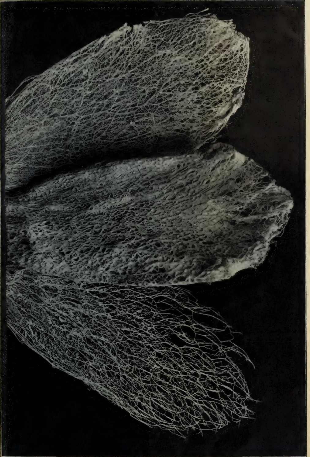
CLEAN WHITE FIBRE FROM THE CACTUS LEAVES FOR CELLULOSE, PAPER, AND VARIOUS OTHER USES
