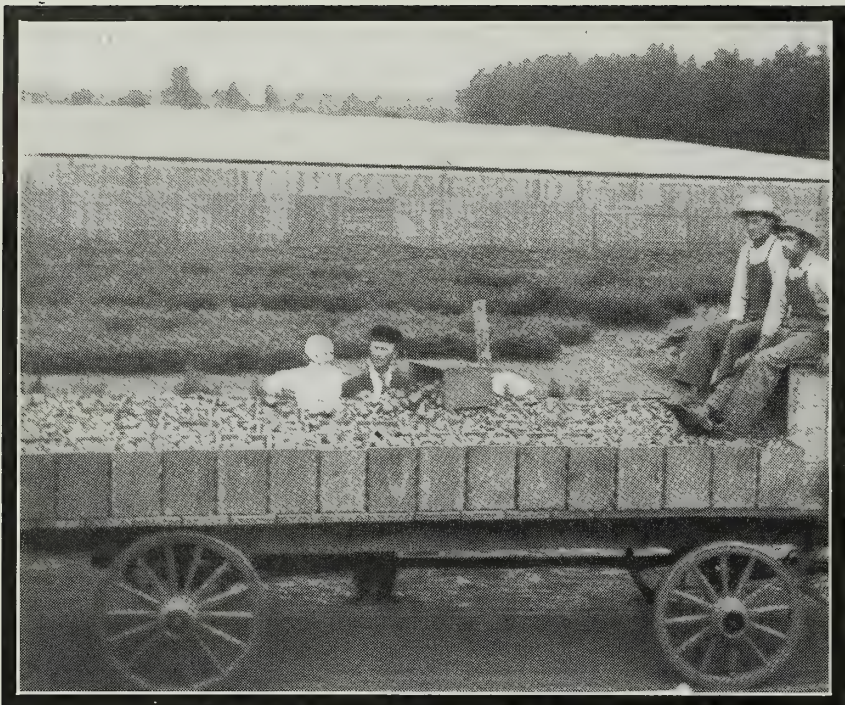
PHOTOGRAPH "E"—Shows one of our low-wheeled wagons with platform which we have found very convenient in hauling the crop from the field into our curing-sheds. The bed of one of these platforms is 16 feet long and 5½ feet wide—just wide enough to hold four rows of crates, or sixty bushel crates, to the load. A platform of this kind can be built very inexpensively, and if you ever use one, you will never try to grow onions in a commercial way without it. "THE GILBERTSON WAY"
