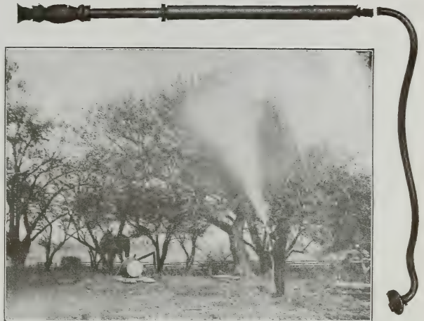
Showing the Standard Pump attached to barrel with 30 feet of hose, enabling the operator to walk around without moving the barrel, covering the entire tree From the Ground without the use of elevated platforms, etc. An ideal orchard sprayer at small cost.
