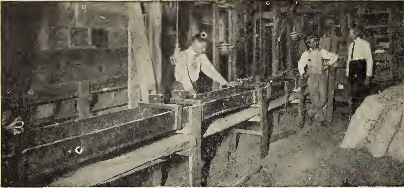
The Far Corn Sorting Belt. The Corn gets its first sorting here, the good ears being picked off from the belt as it goes by and butted and tipped on the revolving wheels shown.
