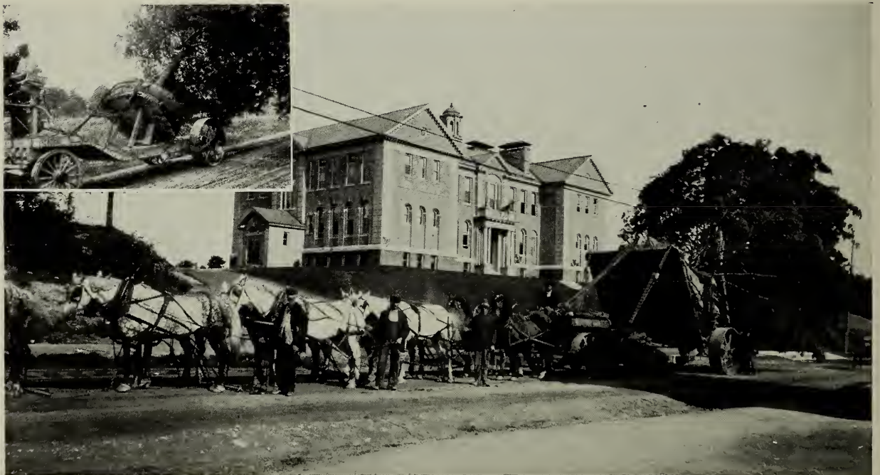
Tree Mover No. 21, all steel. Estimated capacity 30 tons. With this, we can move very large evergreens with a heavier ball than has heretofore been practicable. On the mover is a Pine, 40 years old, 50 ft. high and 40 ft. wide. We have moved several trees of this type and dimension. Are there such trees in your vicinity we can move for you?
