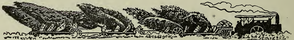
Traction engine and tree movers loaded with Cedars. We have delivered large numbers this way and brought Cedars to the nursery. On one trip as much can be hauled as with thirty horses.
