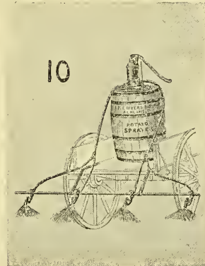
Fig. 10. Four Row Spraying Attachment. No. 1105. Cut shows this attachment as used on an ordinary wagon. We furnish this attachment complete, less barrel, pump and wagon. Mfrs. price, $12.50. Our net price, $8.35
