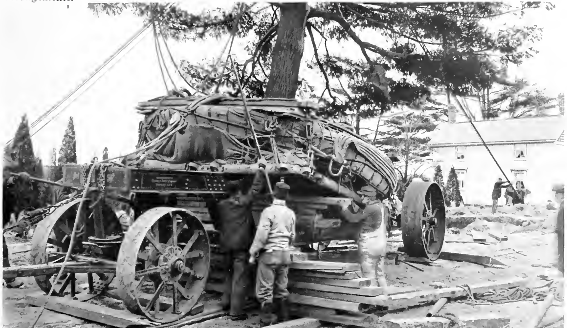
Tree Mover No. 21, all steel. Estimated capacity 30 tons. On the mover is the Pine, illustrated on back cover.
