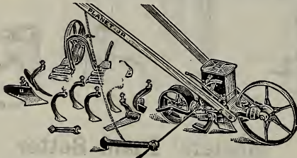
Planet Jr. No. 25 Combined Hill and Drill Seeder and Double Wheel Hoe, Cultivator and Plow.
