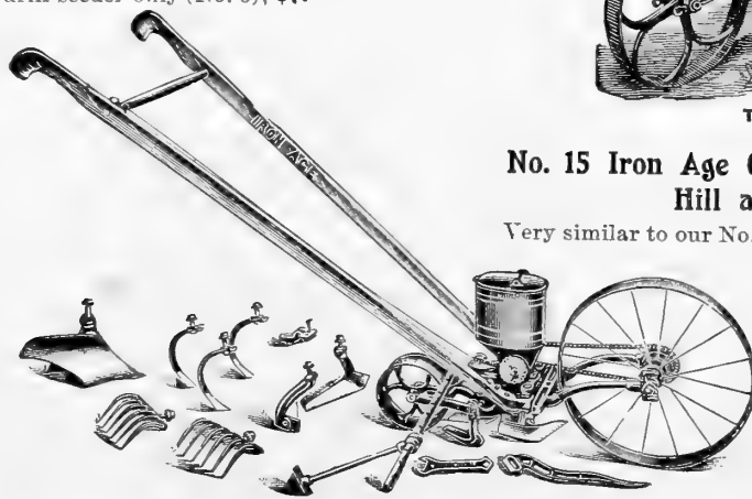
No. 15 Iron Age Combined Single Wheel-Hoe, Hill and Drill Seeder.
