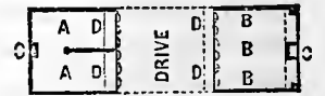
FIG. 2. Fig 2. ground plan of one section of Stable Floor—A. A., horse stables; B. B., cow stables; C. C., manure traps; D. D., mangers.
