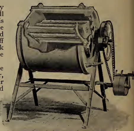
No. 2-H. P. Minnetonna, with part of side and one end cut away to show the position of basket and working roll inside of all Minnetonna models.
