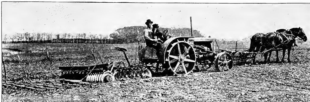
Double Disking and Harrowing at One Operation—Followed up with the Corn Planter—Funk Farms.
