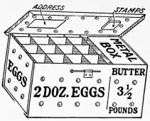
Metal Crate showing compartment for the eggs, shock absorbers that prevent breaking, "opening" in lid for address, and slots to hold stamp card—reversible.
