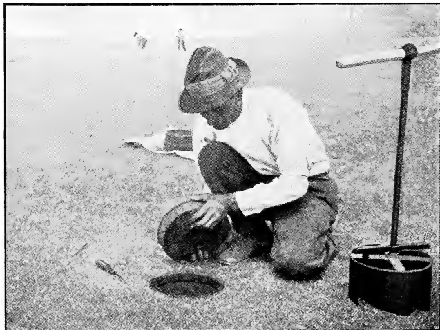
A 10-inch turf repairing Hole-Cutter in use
