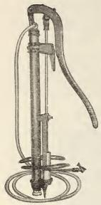
This pump will meet all requirements of a perpendicular barrel pump. It is powerful, light and durable, and will maintain a working pressure of 200 pounds. Has ample capacity for two lines of hose if desired. Because of its high pressure, it is particularly adapted to orchard and vineyard work; also white-washing, cold water paints, disinfectants, etc.
