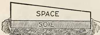
Showing how a coldframe is made Space at highest part 12 in., space at lowest part 6 in., depth of soil 5 in.
