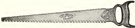
DISSTON PRUNING SAW No. 4 —Duplex, double edge, cast steel blade, polished. Quick acting teeth on one side and plain teeth on reverse edge; beechwood handle, polished; 3 brass screws; 16 inches. Postpaid, $1.35. Not Prepaid, $1.75.
