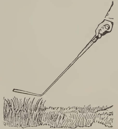
No. 6—LONGHANDLE GRASS HOOK Twelve-inch heavy crucible blade. 43-inch ash handle. Special heavy construction of this hook makes it very serviceable. Each, 85c.
