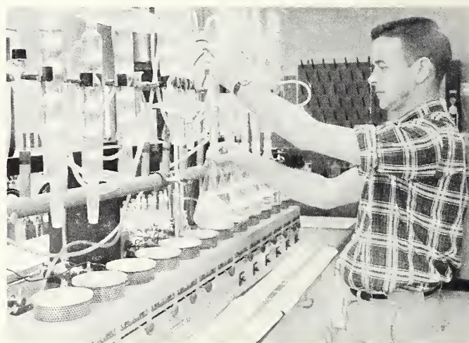
Analytical chemist purifying solvents for use in analysis of insecticide residues.
