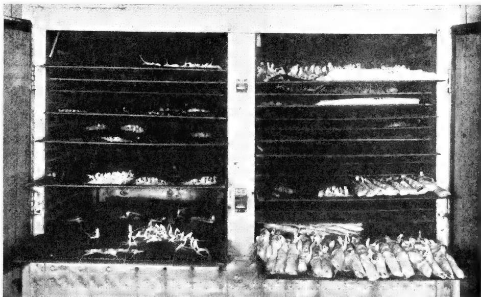
A close up view of one of our seed testers. In these testing machines germination tests are made in the laboratory under ideal conditions. We make corresponding tests in the soil so that we know at all times the correct germination of all seed stocks we have on hand. Seed stocks that are found to be falling in germination and will soon be too low to give a good stand, are immediately removed from our warehouse and distributing plants and are destroyed.
