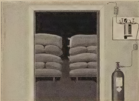
IN VAULT FUMIGATION, Methyl Bromide is introduced from the outside with simple applicator from 1 lb. can or convenient cylinders.
