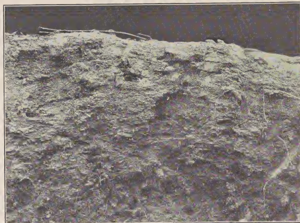
FIGURE 22.—Profile of Leonardtown silt loam, near Washington, D. C., showing detail of lamination in A horizon.
