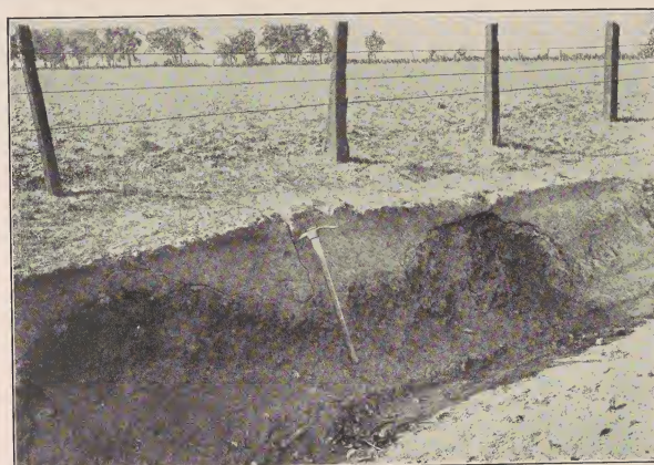
FIGURE 30.—Profile of Susquehanna sandy loam, Milam County, Tex., showing sandy A horizon, heavy clay B horizon, and undulating line of demarcation between A and B horizons.
