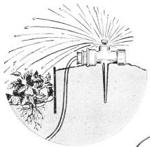
Available with hose attachment. Copper tubing with nozzle is placed in bed before dirt. Special nozzle sprays entire bed. Merely connect hose and turn on. (optional)
