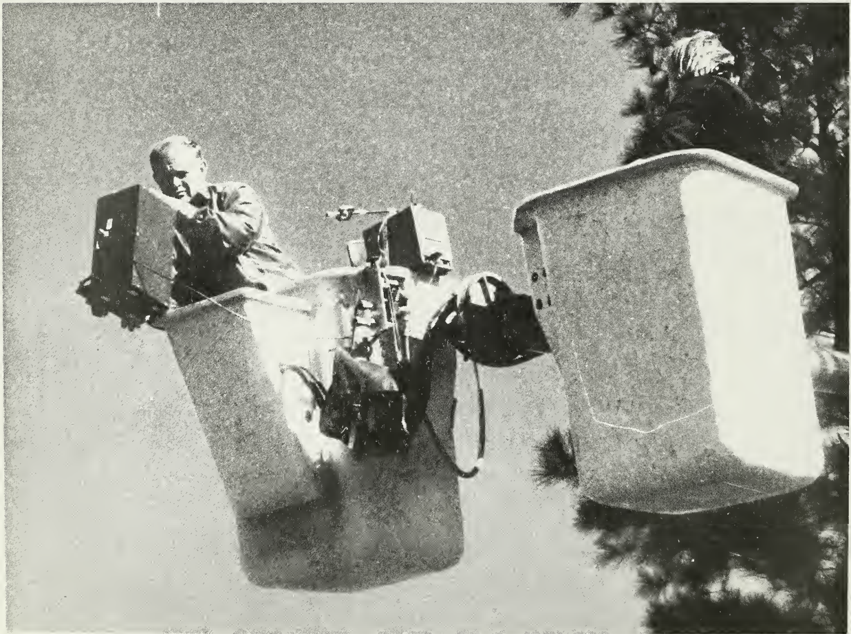
Figure 2. Researcher is shown in a cherry picker above the test site measuring the spectral radiance of vegetation with a 4-channel spectrometer. Ground data were collected as a coordinated effort with the airborne MSS flights to provide baseline calibration data used during multispectral processing.
