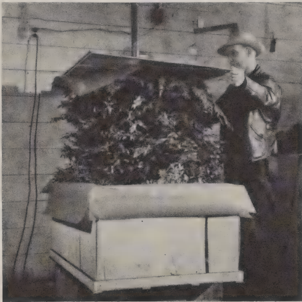
A hydraulic press at the processing plant compresses bunches of evergreen huckleberry in a crate for shipment.
