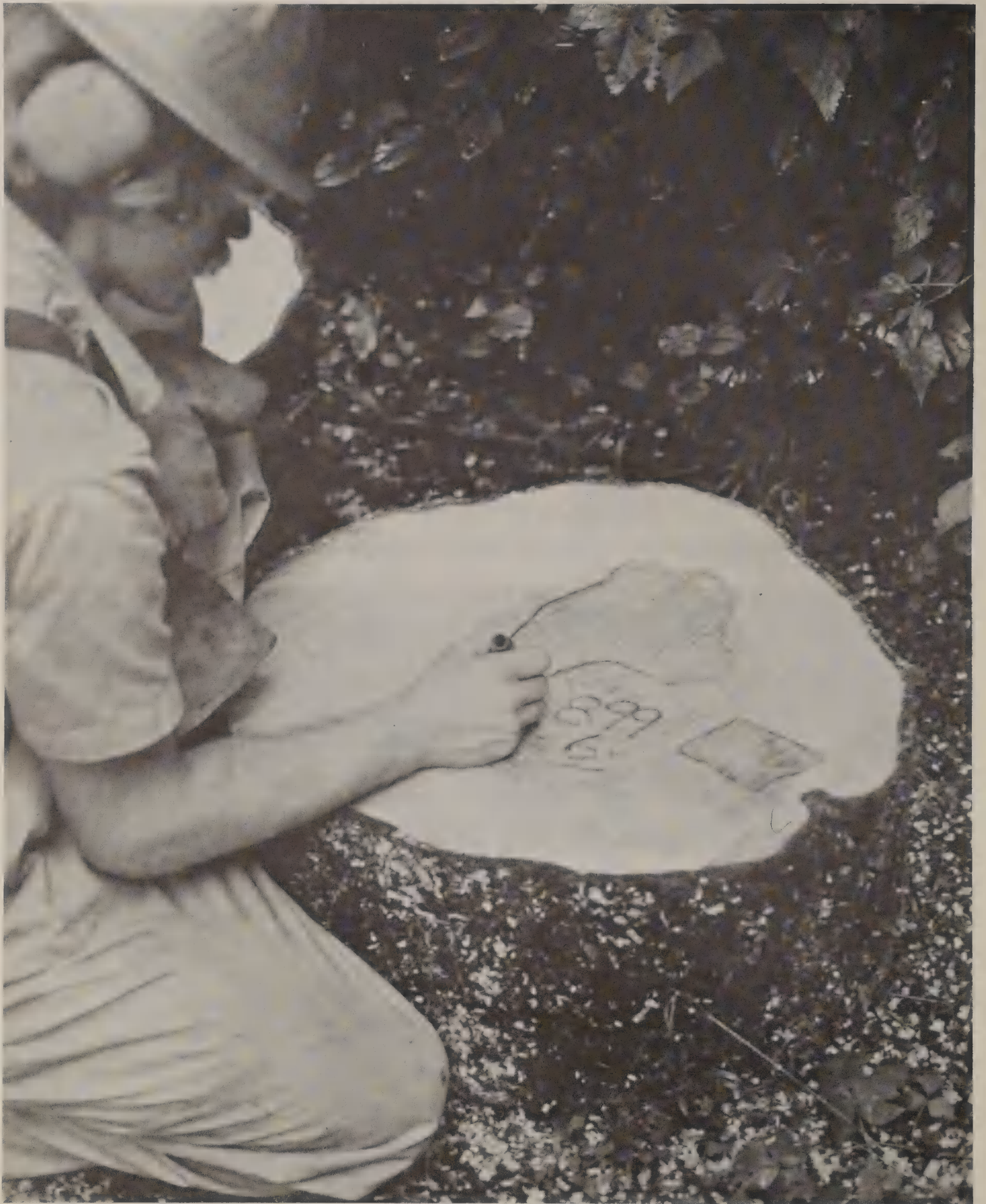
Figure 6. Outlining area of decay on the face of a disk from a decayed western hemlock, Aberdeen, Washington.
