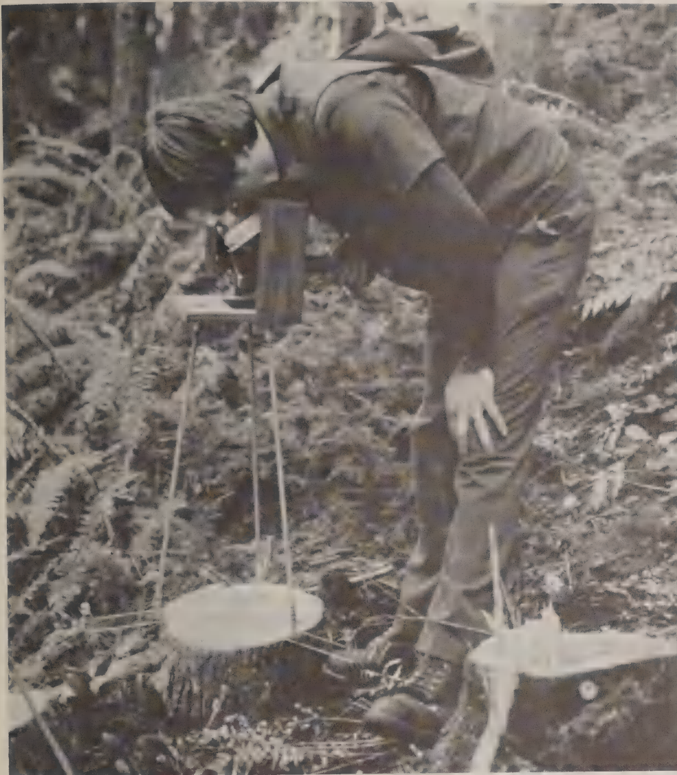
Figure 7. Photographing decay with Polaroid camera on calibrated stand, Bull Run, Oregon.
