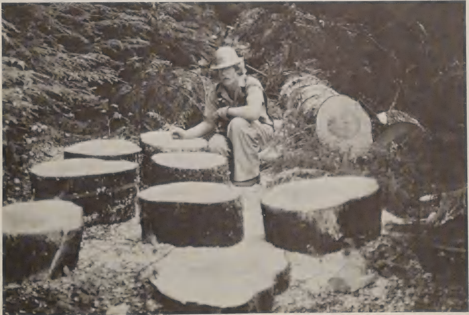
Figure 5. Western hemlock dissected at one foot intervals to the top of an extensive decay column, Aberdeen, Washington.
