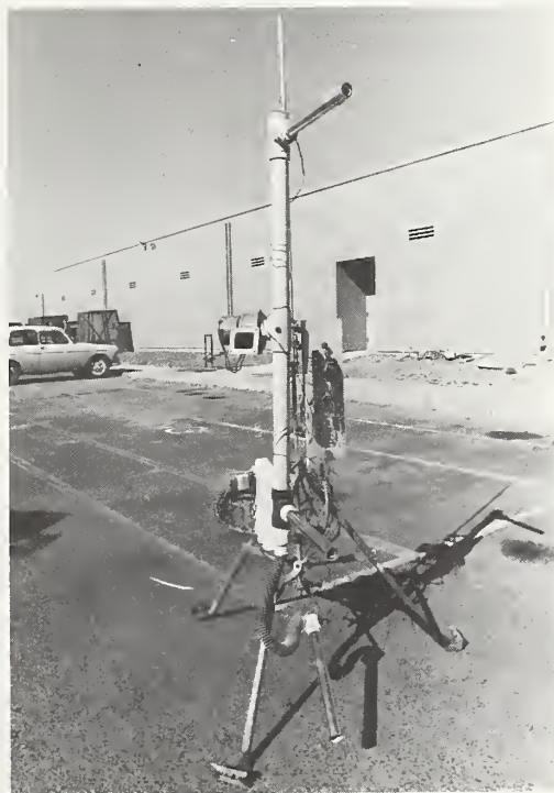
Figure 2.--Sensor stand support for air-temperature manifold and sensor tubes, stepping switch, and terminal board.
