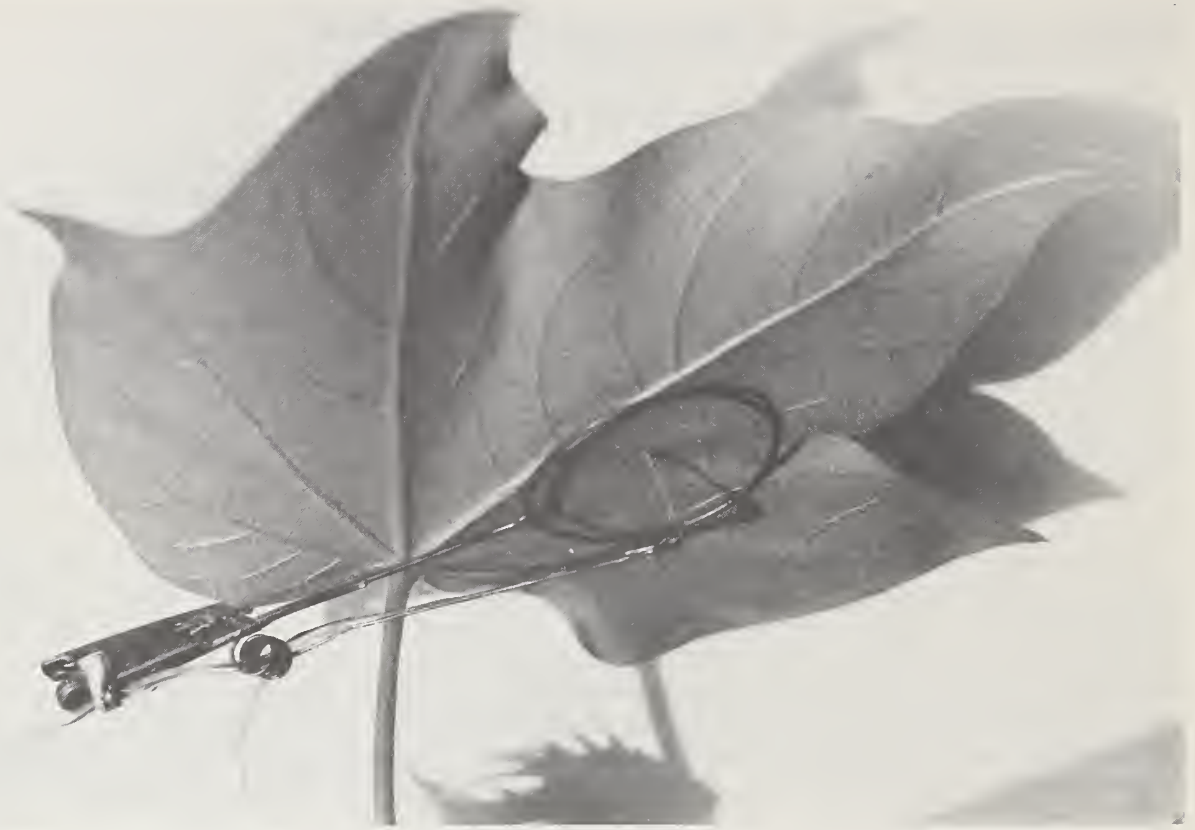
Figure 3.--Thermocouple leaf thermometer on cotton leaf (underside).
