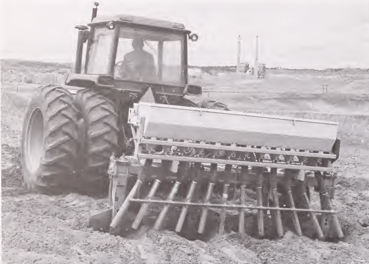
Figure 6.--Hodder gouger makes depressions in soil and simultaneously seeds area to establish plant cover.
