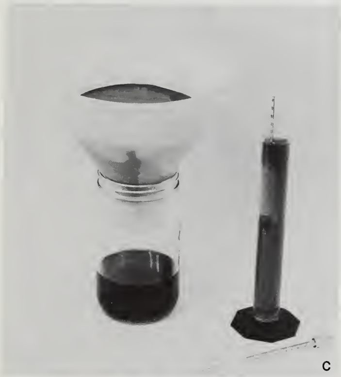
Figure 1.—Equipment for determining salt content: (A) unthickened or low-viscosity retardants; (B) gum-thickened retardants; (C) clay-thickened retardants.
