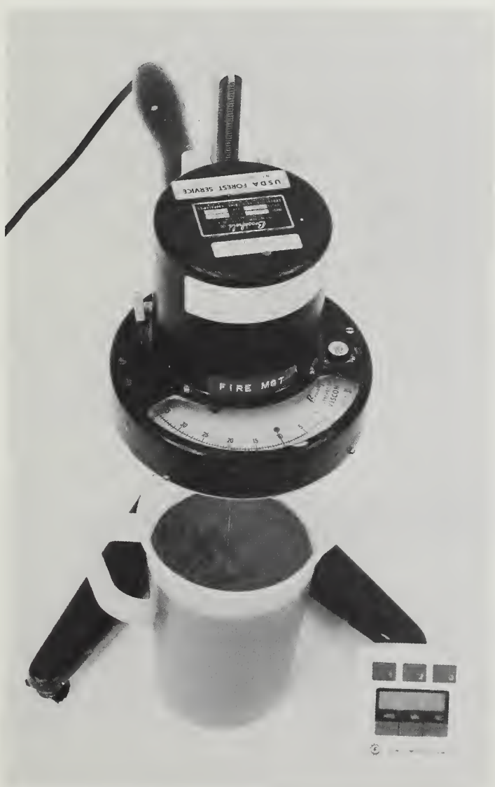
Figure 4.—Brookfield viscometer used to determine retardant viscosity.
