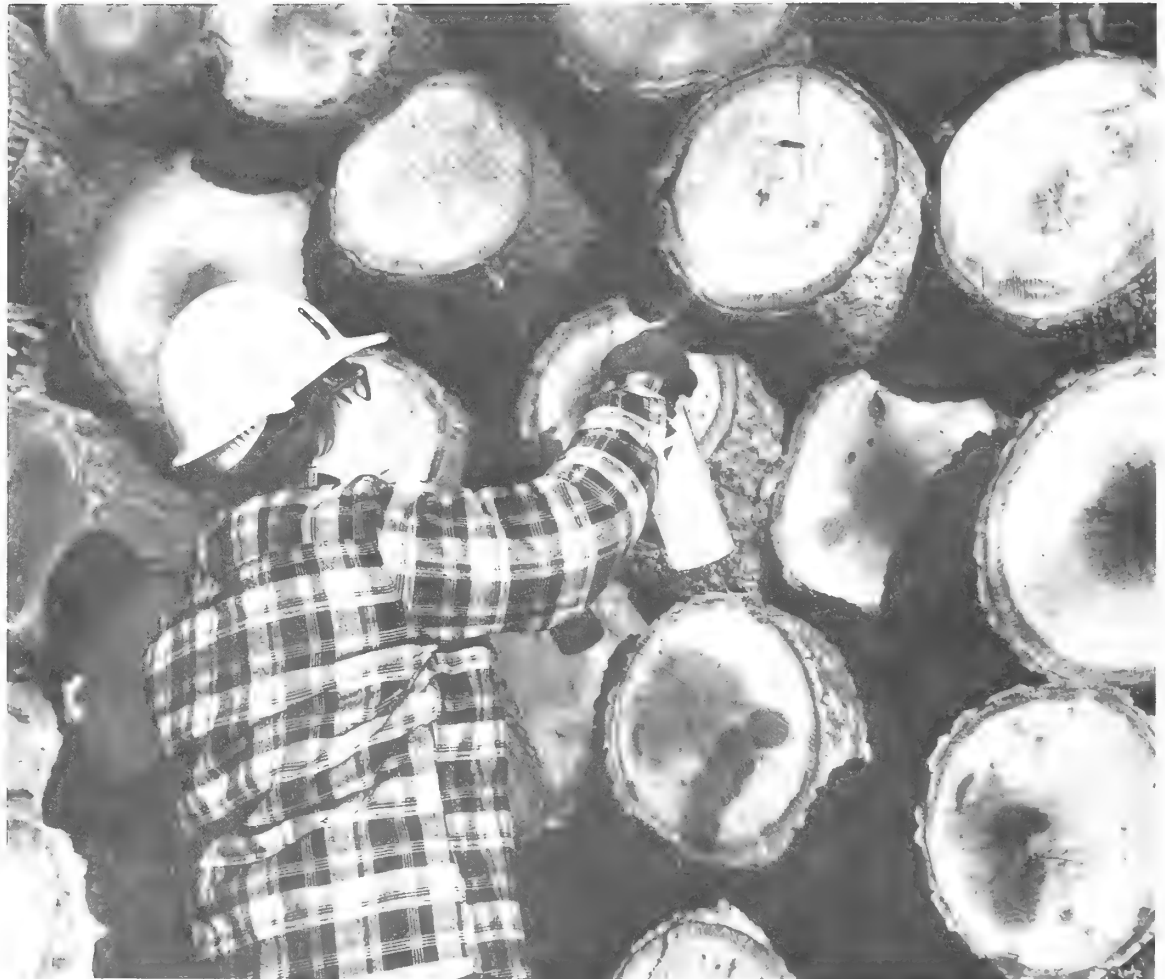
The color change in a sodium nitrite solution sprayed on logs separates red from white oaks.
