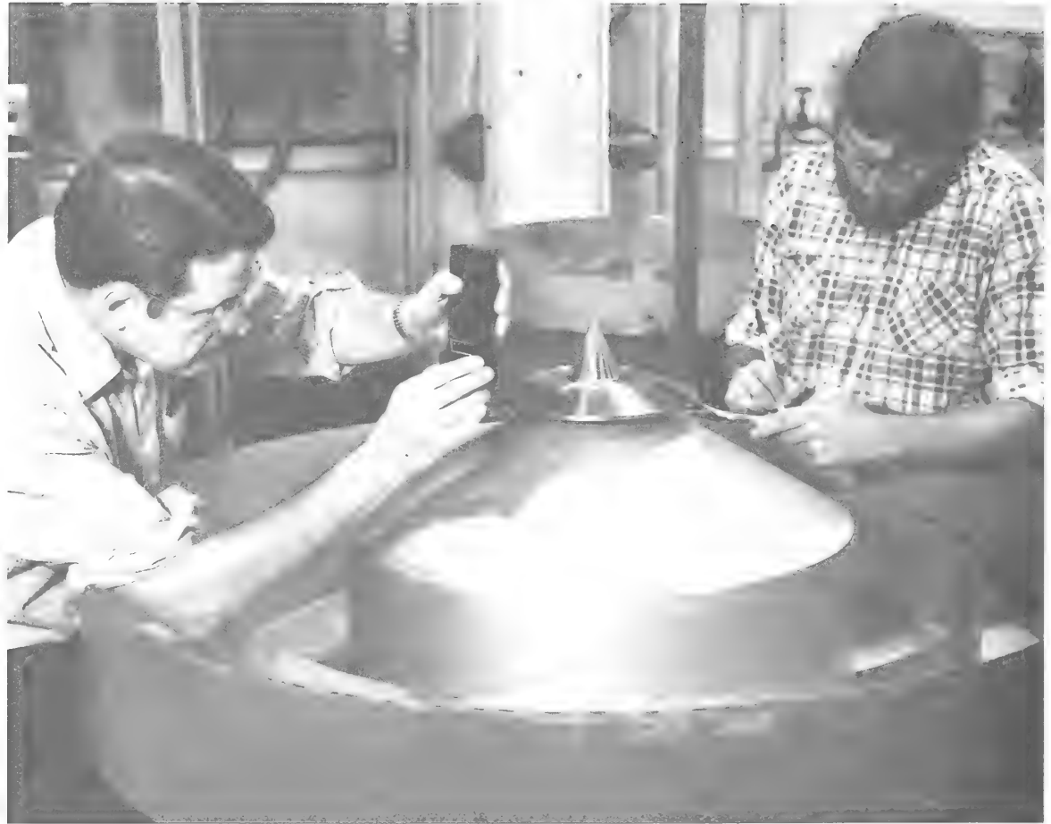
A smooth metal disk spinning at high speed separates particles on the basis of size, density, and wettability.
