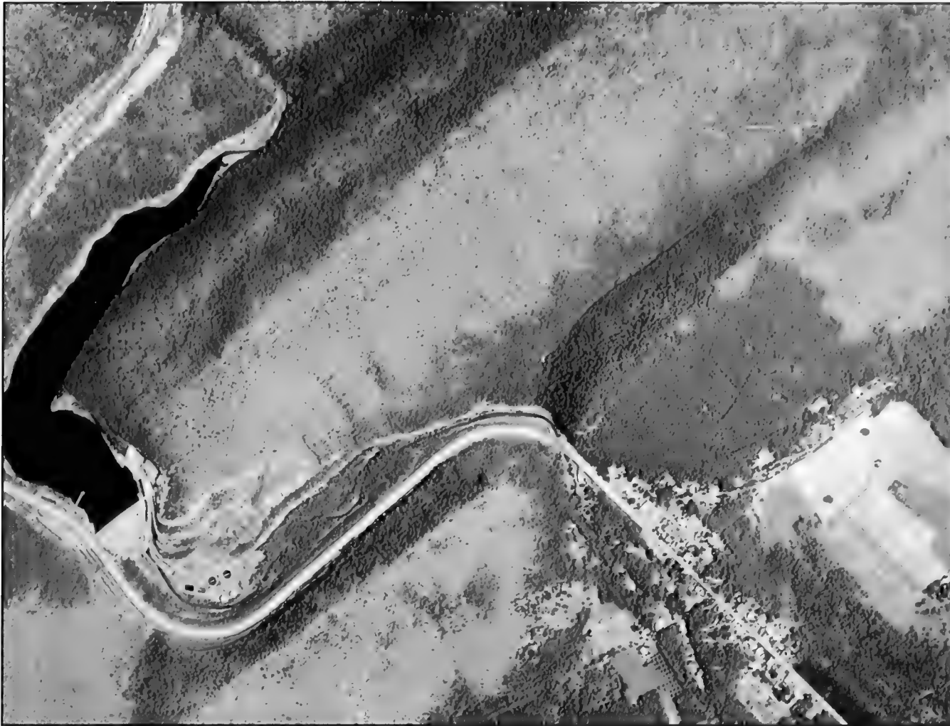
Figure 8. High-altitude infrared photography over Mifflin County, PA. Gypsy moth defoliation appears gray blue; undamaged forests photograph bright red; and water photographs black.
