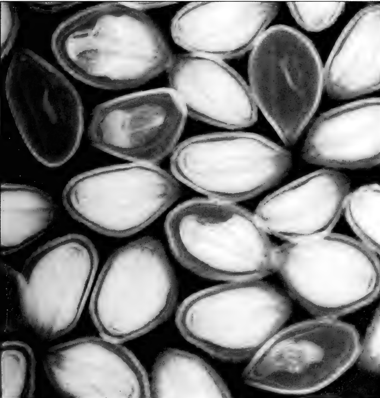
Figure 3. Radiograph of full, empty, and seed bug-damaged seed.
