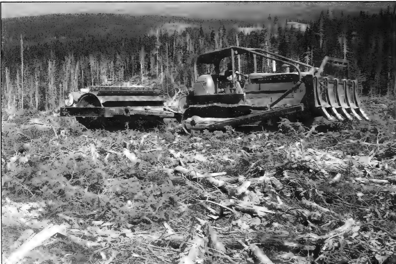
Figure 6. Roller chopping a lodgepole pine clearcut to prepare the site and to destroy infected residual trees.
