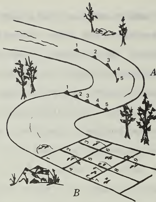
Figure 9. Examples of transect and grid sampling schemes. A illustrates longitudinal and transverse transects while B illustrates a grid of nine sampling sites (after Averett, 1977).
