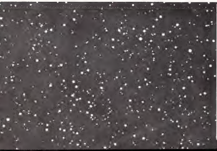
Figure 9.--Spray deposits on one-half of a deposit card placed at plot 2.
