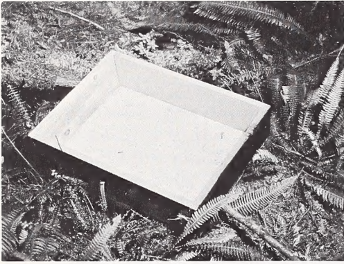
Figure 3.--Ground tray used to collect dead larvae and frass falling from sample trees.
