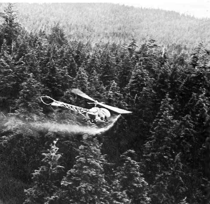
Figure 1.--Helicopter spraying test area with water-based suspension of Bacillus thuringiensis .
