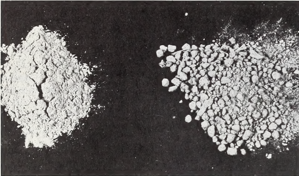
Figure 4.—Volcanic ash (left) and mud (right) (x 2) used in the study. (Note larger particles of mud.)
