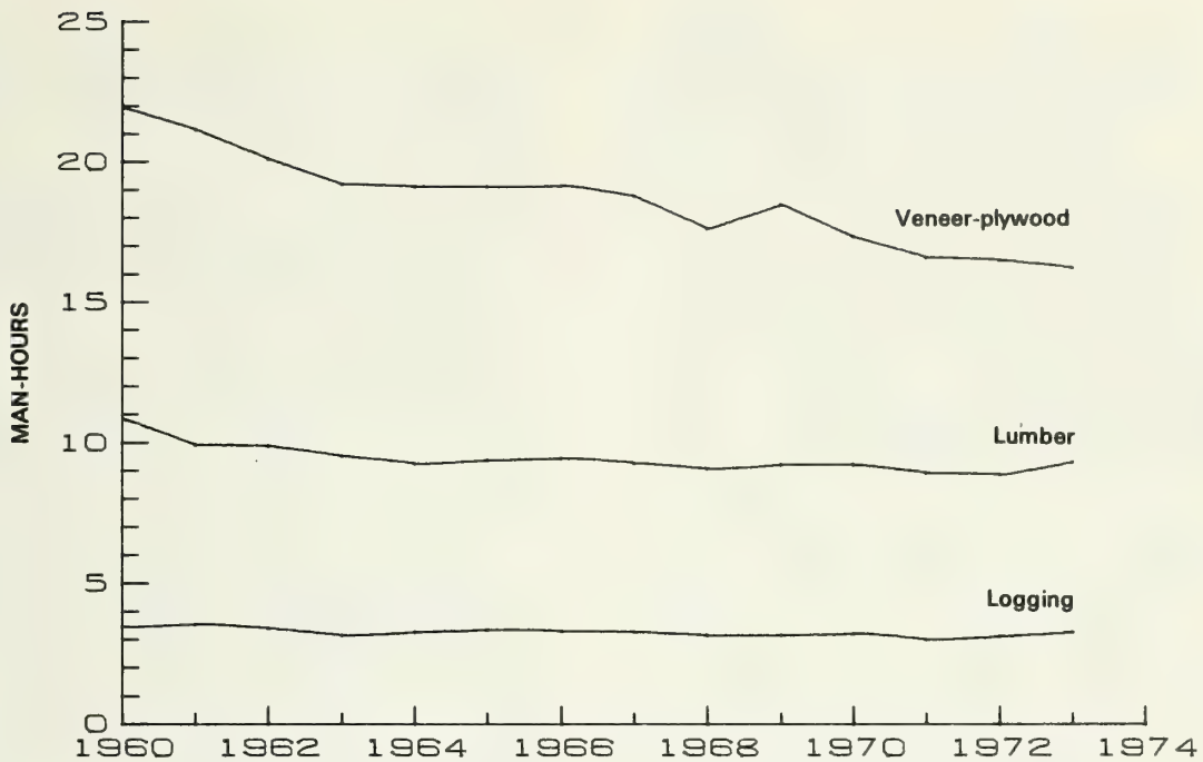
Figure 4.--Man-hours required per thousand board feet of logs processed in the logging, veneer and plywood, and lumber industries in Washington and Oregon, 1960-73. Source: Wall and Oswald (1975).
