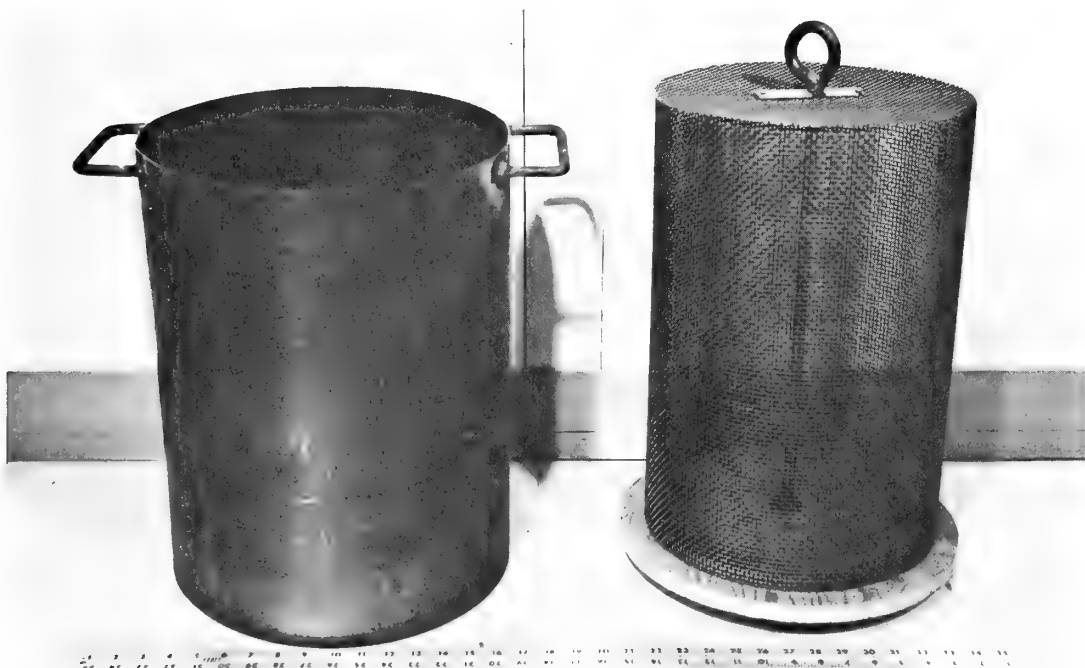
Figure 6.--Basket used as artificial "redd" and outer casing for retaining sediment when basket was removed from streambed.
