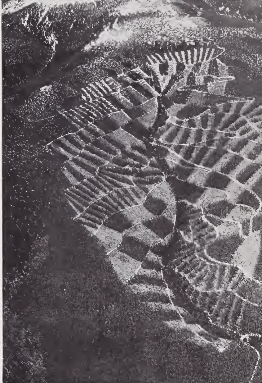
Figure 3.--Timber cutting pattern and road system on Fool Creek experimental watershed. Annual sediment accumulation is measured in the debris basin at the lower right-hand corner of photograph.
