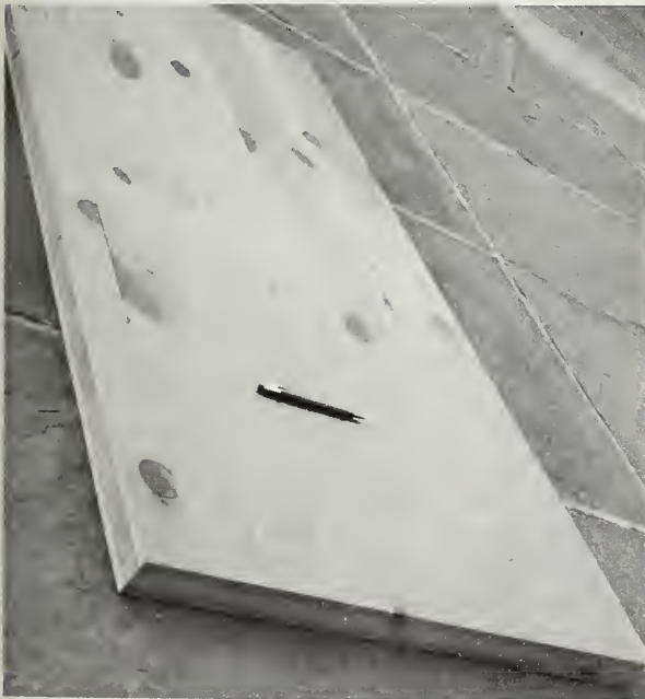
Figure 1.--Test panel with resawn 4/4 lumber faces glued perpendicularly to the nominal 1-inch core boards.
