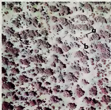
Figure 3.--One hundred percent correct identification of small juniper (a), mountain mahogany (b), and pinyon pine (c) is possible on the color infrared photos (left) at 1:1,200 scale, exposed in July or August. These species are frequently misinterpreted on color photos (right) at the same scale.
